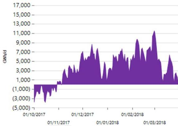
Figure 32 - UGS injection/withdraw profile. Winter 2017/2018
