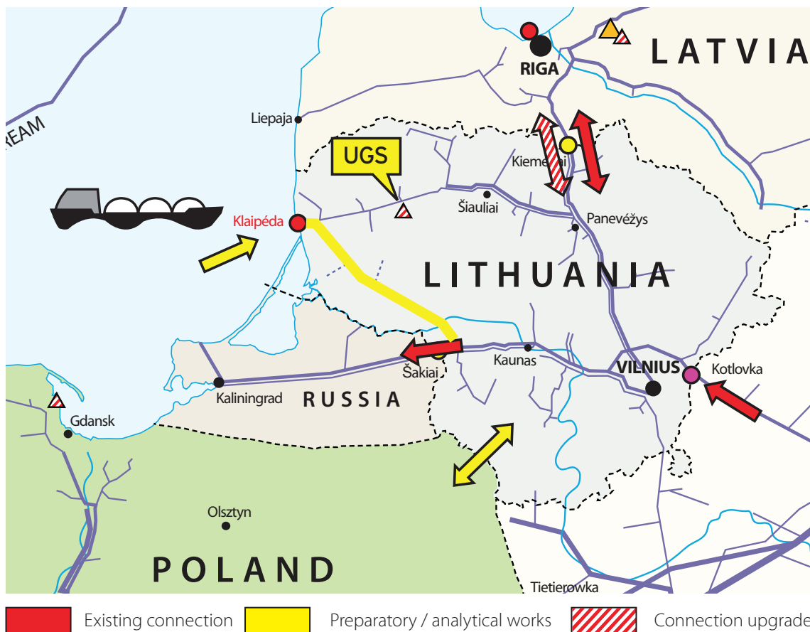
Figure 27: Existing and planned gas infrastructure in Lithuania. Source: Lietuvos Dujos
