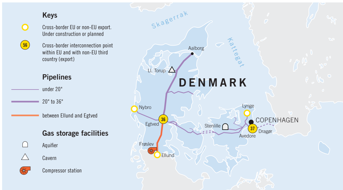
Figure 2.25: The Danish gas production, storage and transmission system
