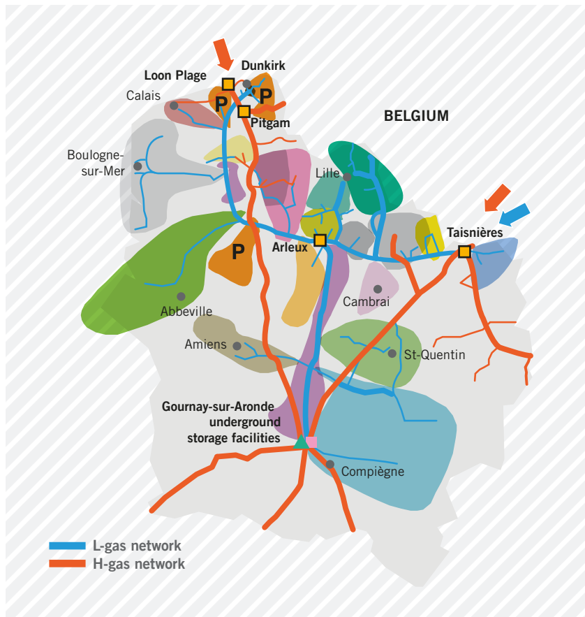
Figure 7.10: Clustering of L-gas conversion process (Source: GRTgaz)
