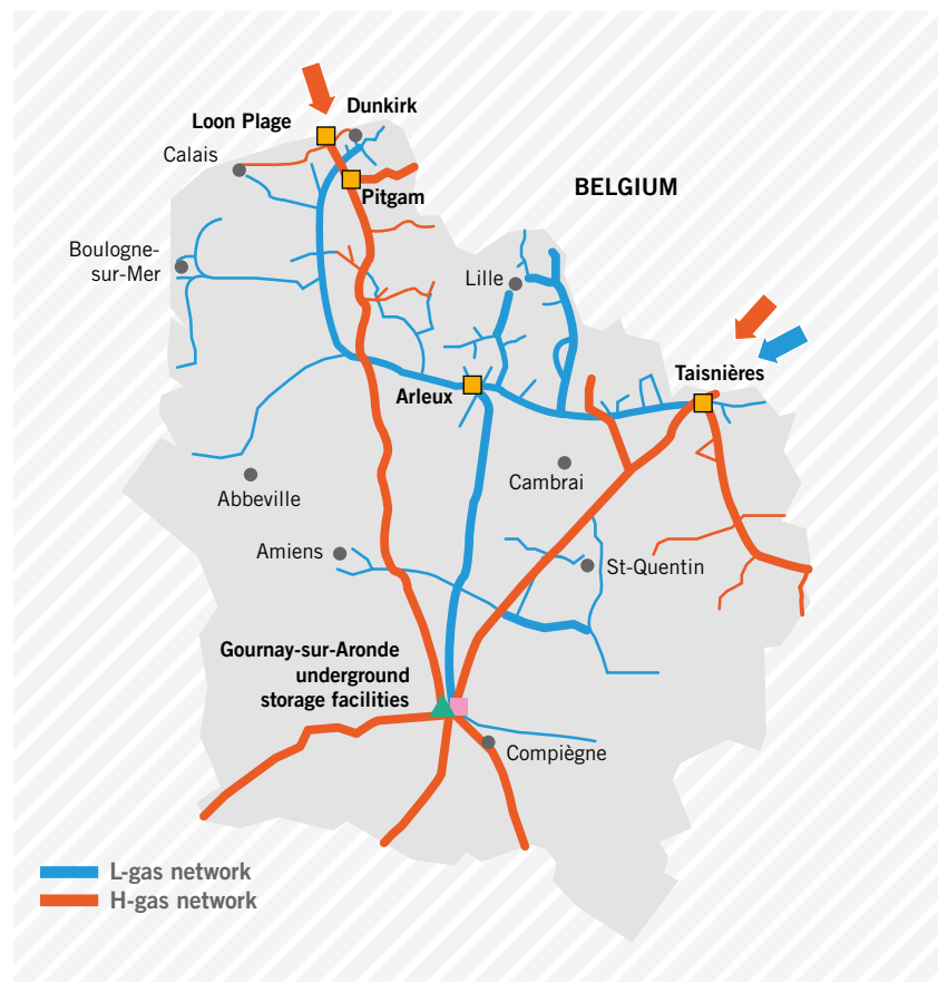
Figure 7.9: L-gas and H-gas networks in France (Source: GRTgaz)
