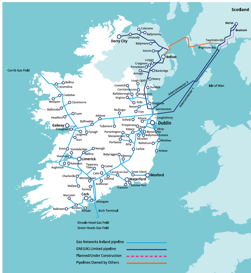
Figure 9.9: Ireland & Northern Ireland Transmission pipelines (Source: Gas Network Ireland Network Development Plan 2016)
