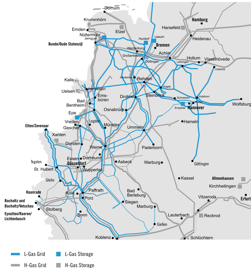
Figure 7.5: L-gas transmission network Germany (Source: TSOs Germany)
