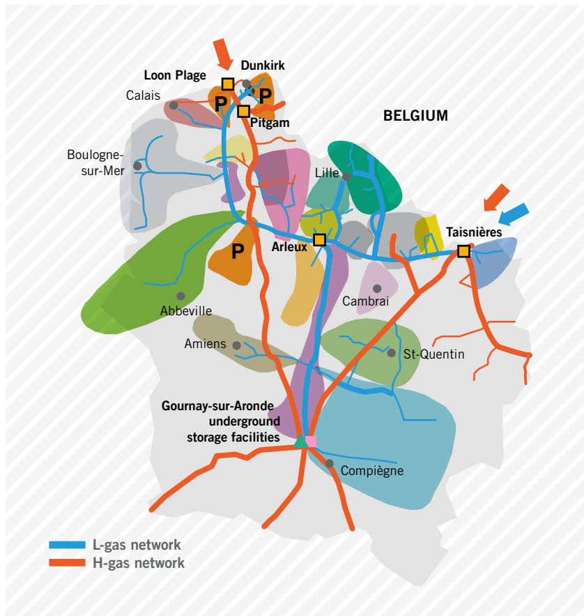
Figure 7.10: Clustering of L-gas conversion process (Source: GRTgaz)
